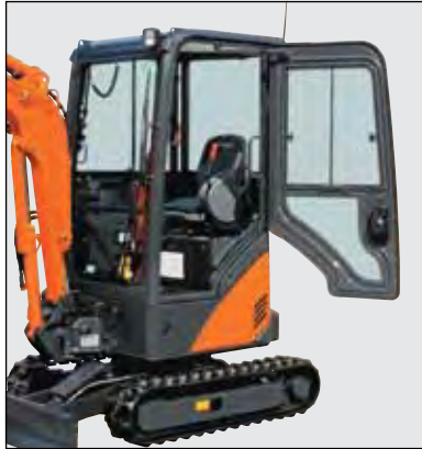
Door Opening Lock System (Cab equipped machines)
