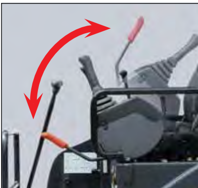
Lock Lever Allows Lock/Neutral Engine Starting
